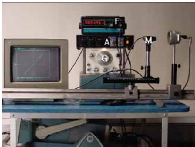
Fig. 1. Apparatus used in the measurement of the speed of sound using Lissajous figures.
